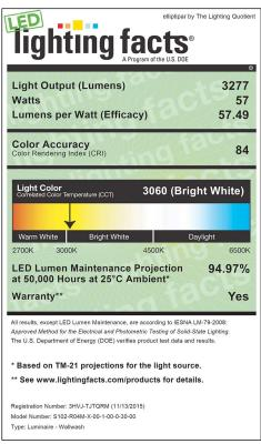
"M" light output is 819 lm/ft (700 mA), 14 W/ft. based on a 4ft fixture.
